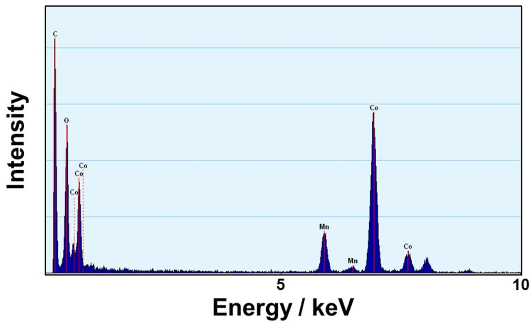
**Figure S1.** EDX spectrum of the MCO@RGO composites.
