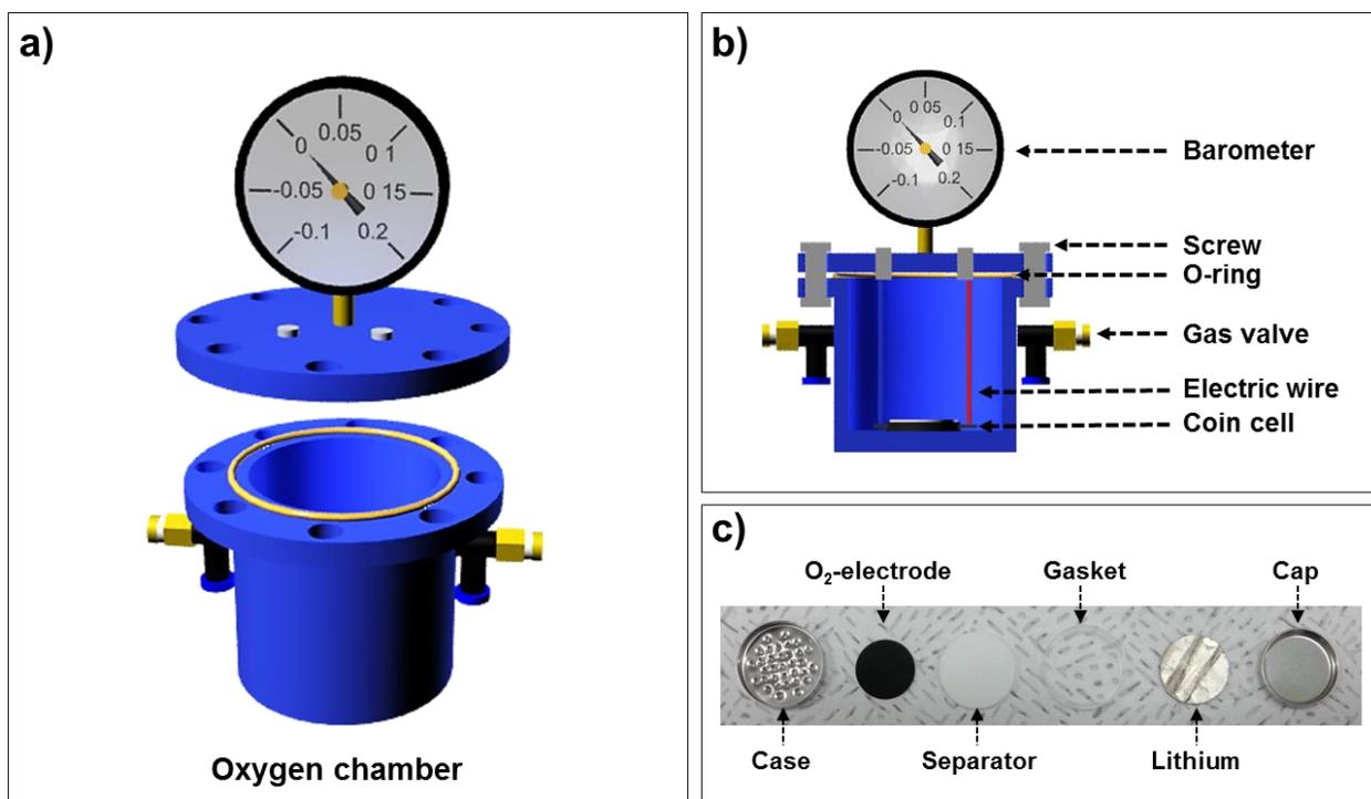
**Figure S4.** (a) Illustration of oxygen chamber of Li-O<sub>2</sub> cells. (b) Cross-sectional scheme of assembled Li-O<sub>2</sub> cells. (c) An optical image of coin cell components used in this study.
