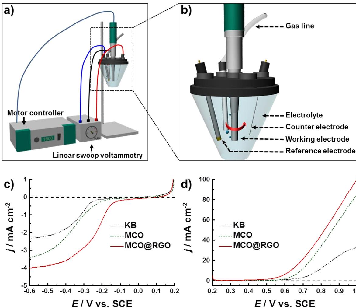
**Figure S3.** Illustration of the LSV and RDE used for the demonstration of ORR/OER activities of the as-prepared catalysts. LSV profiles of (c) ORR and (d) OER for KB, MCO NWs and MCO@RGO composites in (c)  $\text{O}_2$ -saturated and (d)  $\text{N}_2$ -saturated 0.5 M aqueous NaOH electrolyte at a scan rate of  $10 \text{ mV s}^{-1}$  with a rotating speed of 1600 rpm.
