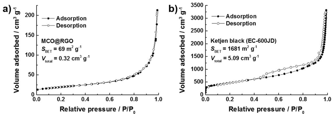
**Figure S9.**  $N_2$  adsorption/desorption isotherms of (a) the MCO@RGO composites and (b) the KB.
