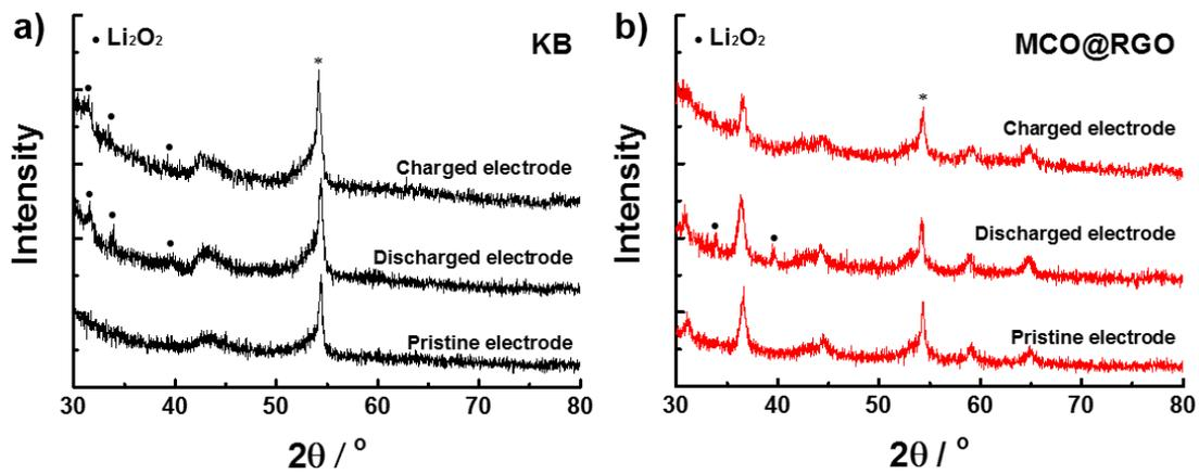
**Figure S8.** XRD patterns of the electrodes with (a) KB and (b) MCO@RGO at different discharge/charge stages. Peaks marked with asterisks derive from the carbon paper.
