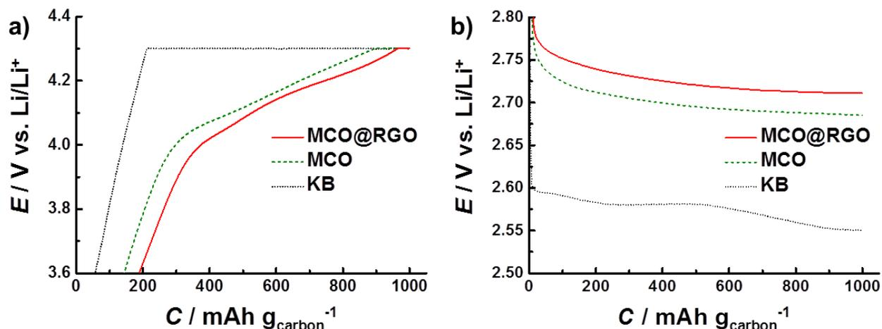
**Figure S6.** Magnified voltage profiles for (a) first charging and (b) first discharging of the Li-O<sub>2</sub> cells with KB, MCO NWs, and MCO@RGO composites at a current density of 200 mA g<sub>carbon</sub><sup>-1</sup> in a potential window between 4.3 and 2.3 V under capacity limit of 1000 mAh g<sub>carbon</sub><sup>-1</sup>.
