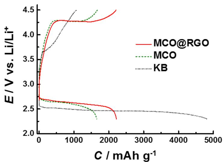
**Figure S5.** The first discharge-charge profiles of Li-O<sub>2</sub> cells with KB, MCO NWs, and MCO@RGO composites. The capacities are normalized by the total mass of electrode (carbon + binder + catalyst).
