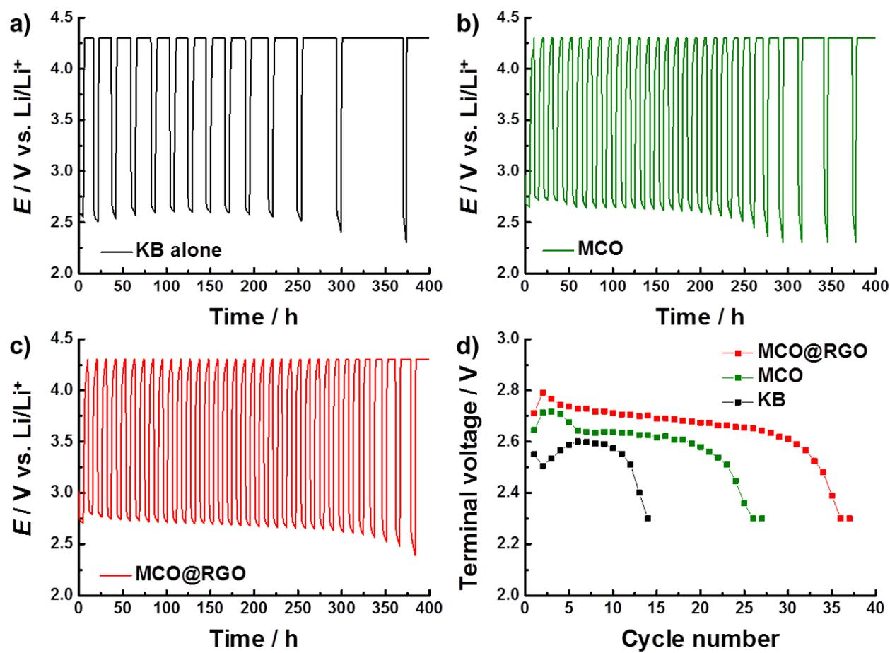
**Figure S7.** Potential-time curves of Li-O<sub>2</sub> cells with (a) KB, (b) MCO NWs, and (c) MCO@RGO composites. (d) Plot of terminal voltage as a function of cycle number.
